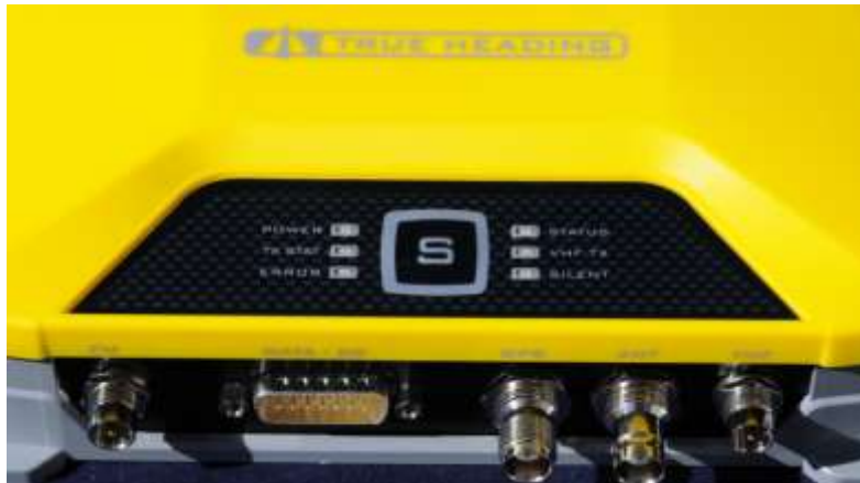
Figure 7 AIS-CTRX CARBON + connectors. From the left FME (Female) for FM radio (a 1,6 m prepared cable comes with delivery), 15 pole d-sub connection (Male) for data and DC power supply, TNC (Female) for GPS antenna, BNC (Female) for VHF antenna (a BNC to UHF adapter is provided if required. We do however recommend to use a BNC connector direct on the VHF antenna cable. Finally to the right a FME (Female) connector for the VHF radio (a 2 m prepared cable comes with delivery).
