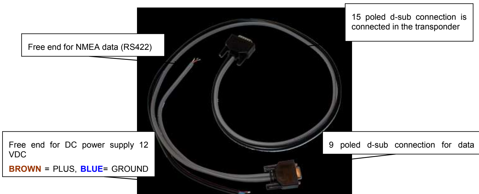
Figure 9 AIS-CTRX CARBON data and DC cables
